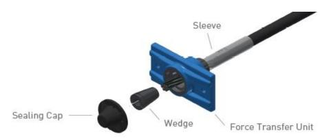
The XU2 system covers the whole anchor assembly comprising the coated steel force transfer unit, the steel wedge, the plastic sleeve, the plastic nut and the plastic sealing cap.
